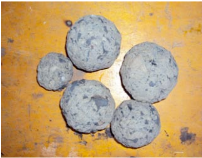
Samples of hand made briquettes: doughnut shaped Components: charcoal dust and waste paper mixed in haphazard manner
