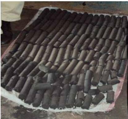
Sample briquettes from motorized screw press Rod-shaped. Components: charcoal dust with 3% of clay added as a binder
