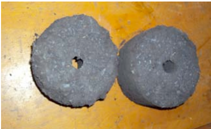
Samples of piston pressed briquettes: cylindrical shaped, hollow in the middle. Mixing ratios: charcoal dust: paper 2:1
